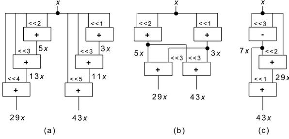
Fig. 2. Shift-adds implementations of  $29x$  and  $43x$ : (a) without partial product sharing [7]; with partial product sharing: (b) the algorithm of [3]; (c) the algorithm of [6].
