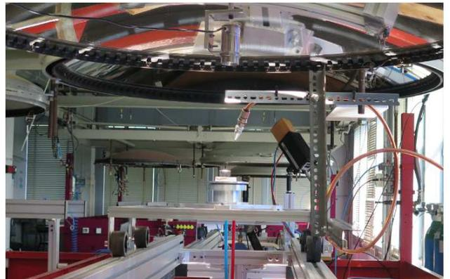
Fig. 2. Visualization the 900W solar furnace at PROMES with a SiC sample on the testing table. The air flow nozzle for active cooling is above (away) the sample. The sun light is guided by a heliostat at the ground level to the parabolic mirror that concentrates the light. A pyrometer located near the parabolic mirror measures the temperature of the sample.
