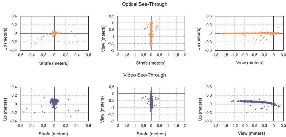
**Figure 3:** Error distribution around target separated by axis. OST in orange and VST in purple.
