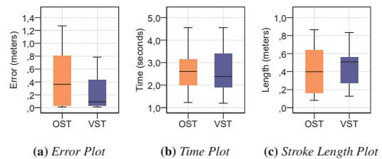
**Figure 4:** Task performance - median, first and third interquartile ranges (boxes) and 95% confidence interval (whiskers) for error, time and stroke length. OST in orange and VST in purple.
