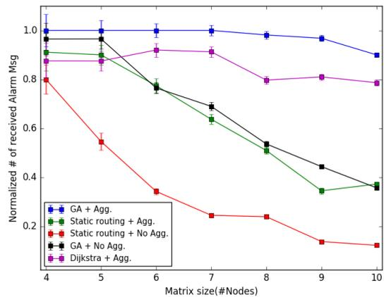
Fig. 5. Message delivery ratio, with the sink at the center of the grid.
