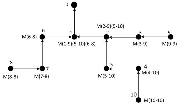
Fig. 2. Network topology of WSN, showing data message aggregation process.
