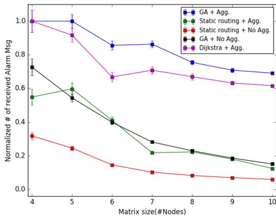
Fig. 4. Message delivery ratio, with the sink at the corner of the grid.
