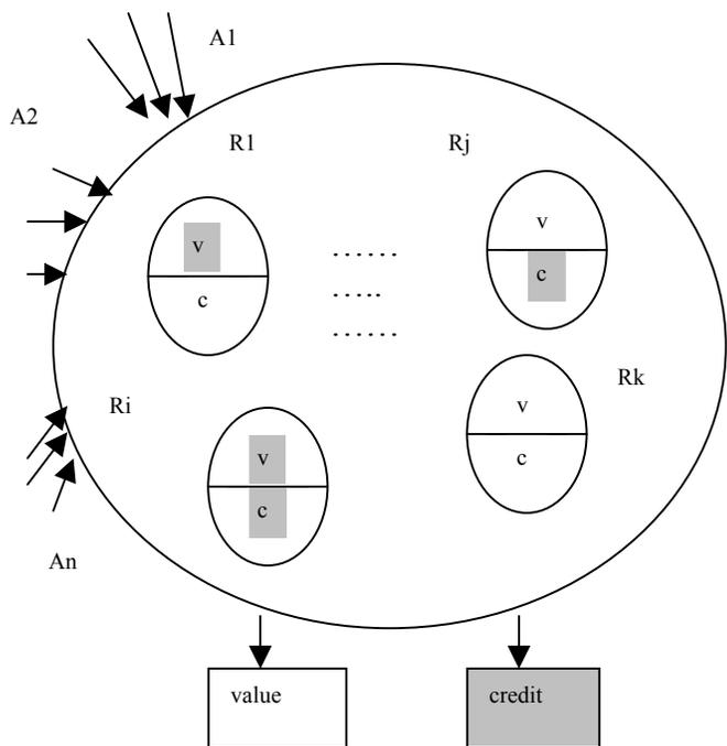
Fig. 1 Internal structure of a Neuron-Value and Credit bits
