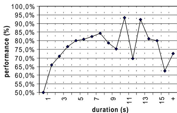
Figure 4. Evolution of the identification rate with utterance duration.
