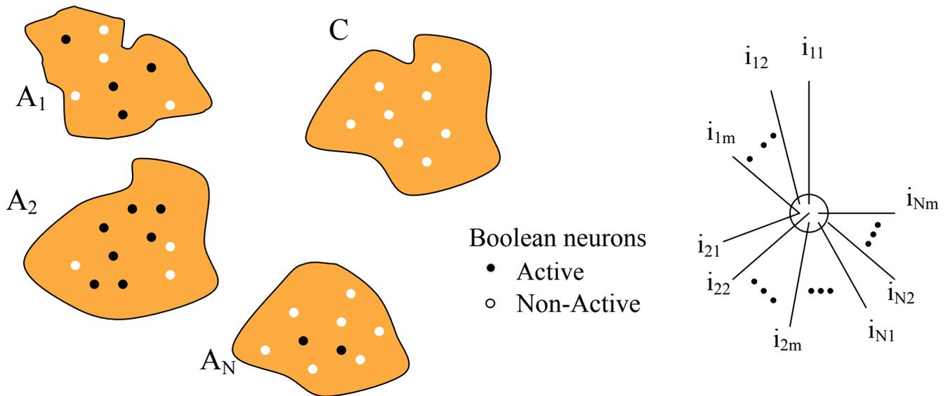
**Figure 1 – FBN Areas and Individual Neuron Structure:** neurons are binary entities grouped into areas (or concepts); the value of each concept is given by the ratio of active neurons; each neuron has  $m \times N$  inputs that can randomly sample the value of  $m$  neurons from each of  $N$  antecedent concepts
