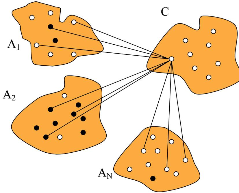
**Figure 2 – Inference of a single Neuron in a FBN:** In this example, the neuron samples  $m=3$  neurons in each of its  $N$  antecedent areas and counts how many of those neurons are active in each area. The combinatorial combination of the counts will be compared to a stored (previously learned) value that indicates if the neuron should or not be activated.
