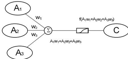
Fig. 2. Concept inference scheme on a FCM.
